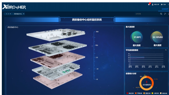
Fig. 3 Main interface of power environment monitoring system
