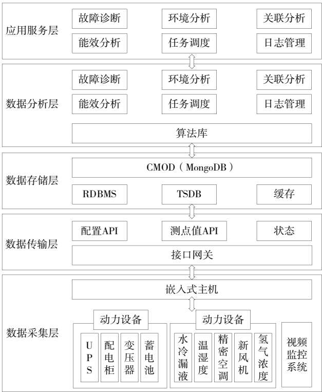
Fig. 1 Logical architecture of power environment monitoring system 图 1 动环监控系统逻辑架构
