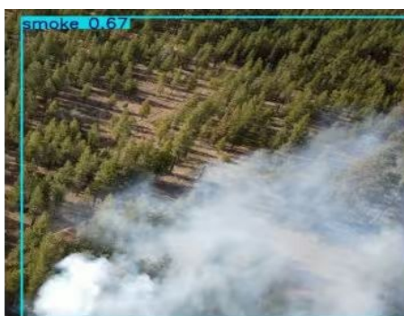
(f) YOLOv8n model for smoke detection
