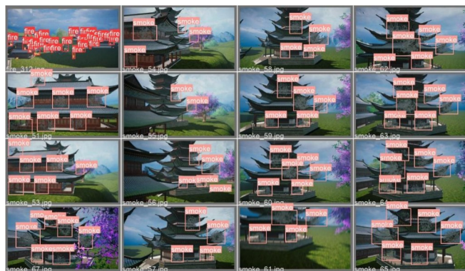
Fig. 11 Detection performance of YOLOv5s-STI on simulated data for flames and smoke
